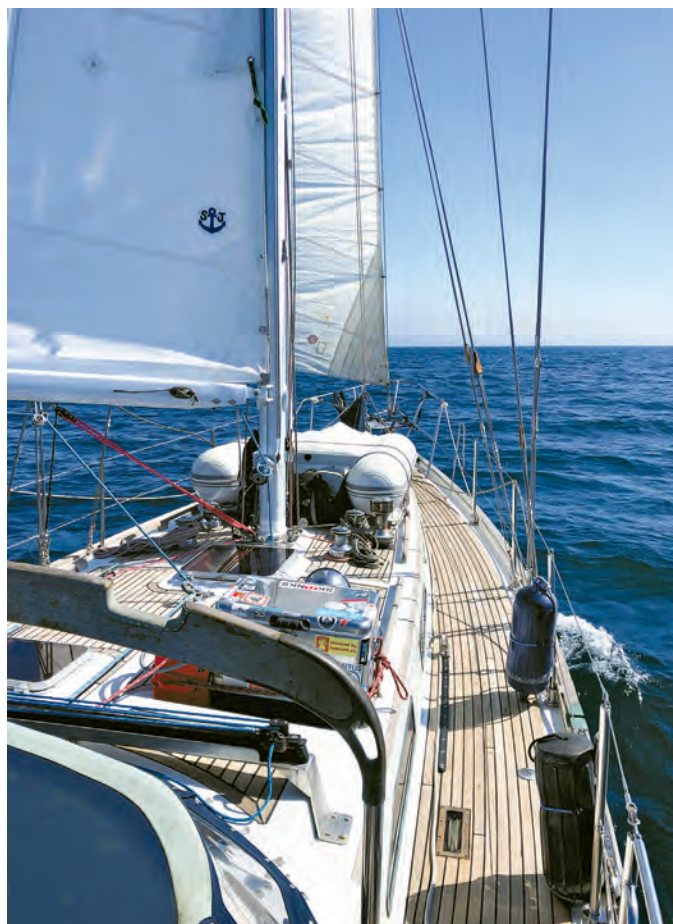
The teak decks and cabintop, typical of most Passport 42s that were built in Taiwan, often need repair after 40-plus years, at top left. Photo courtesy of Two the Horizon Sailing, @twothehorizon.
